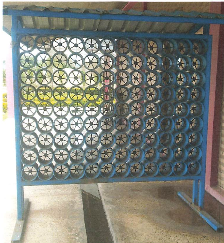
Figure 1: Test wall for exposing EaveTube nettings in a semi-field condition within ATRC compound.
